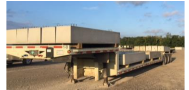
Slabs loaded for delivery.
