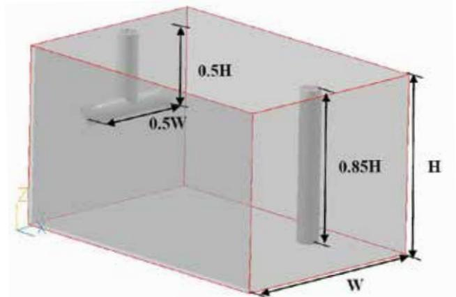
This comprehensive study also shows that local fluid velocities could be reduced by distributing the flow across a larger cross-sectional area. Ideally, the area would occupy the entire cross-section of the of the grease interceptor (i.e., depth multiplied by height), as this setup would provide the lowest fluid velocities. To achieve this, the influent baffle would have to be designed to distribute the incoming flow (Figure 3).
